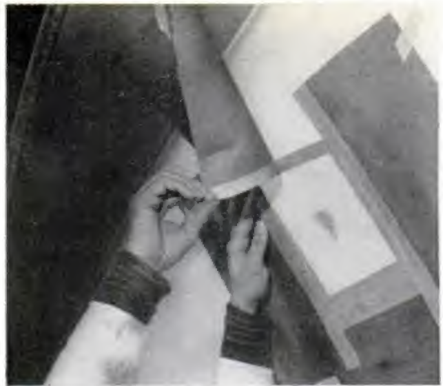
MASKING can be done before or after sanding the repair patch. It's necessary to avoid affecting adjacent areas, especially if gel coat is applied by spray
